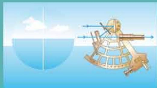
1. Sextant is pointed towards the horizon (where sea and sky appear to meet). A swinging post – the index bar – can be moved along a curving scale marked with angles.
