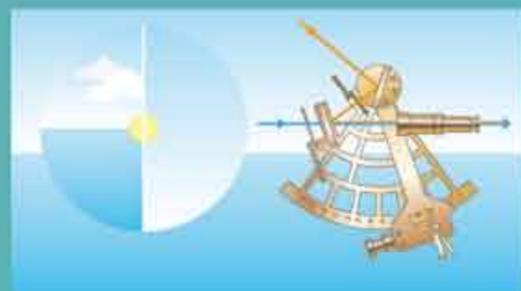
2. As the index bar is moved, the image through the viewfinder splits in two and the Sun is brought down to the horizon. The angle can be read off the curved scale and converted into the altitude of the Sun above the horizon.
